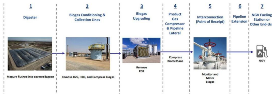
Figure 1: Process to Convert Dairy Biogas into R-CNG
